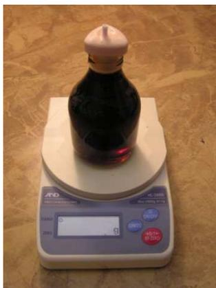
Figure 2 – Pycnometer with a dark beer sample on the scales
