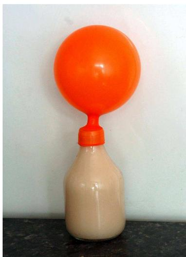
Figure 4 – Inflatable balloon on the pycnometer neck
