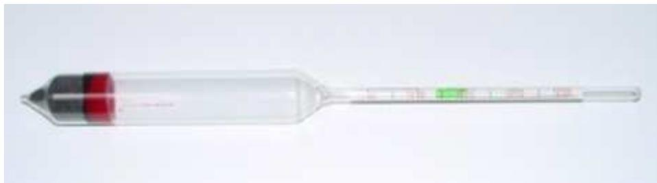
Figure 3 - Hydrometer
