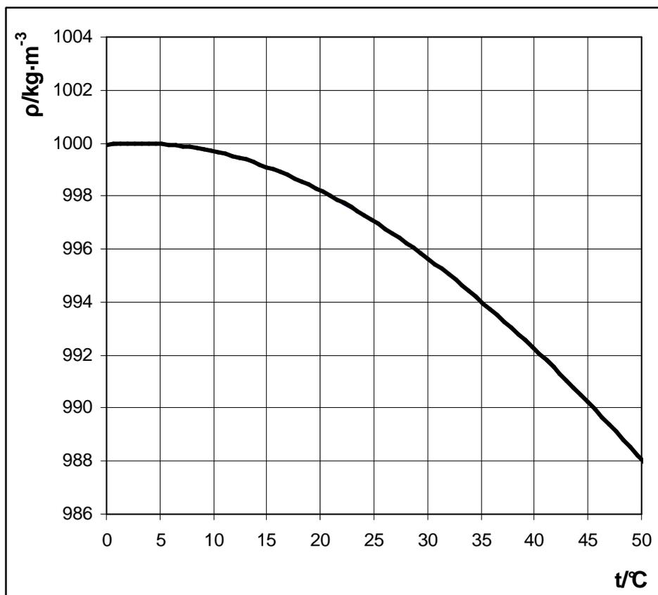
Graph 1 – The dependence of the density of distilled water on temperature
