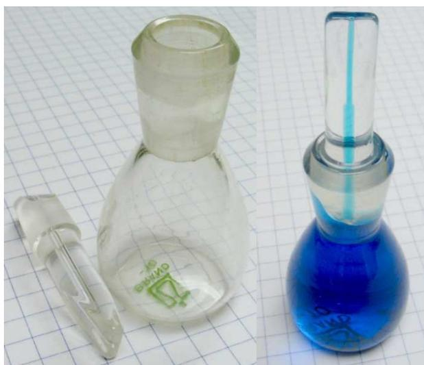
Figure 1 - Pycnometer (Source: Wikimedia Commons)
