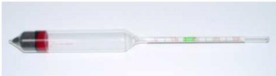
Figure 3 - Hydrometer
