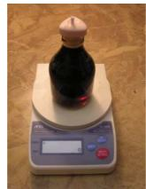
Figure 2 – Pycnometer with a dark beer sample on the scales
