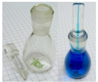
Figure 1 - Pycnometer (Source: Wikimedia Commons)
