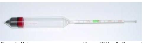
Figure 3 - Hydrometer
