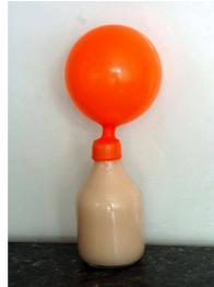
Figure 4 – Inflatable balloon on the pycknometer neck
